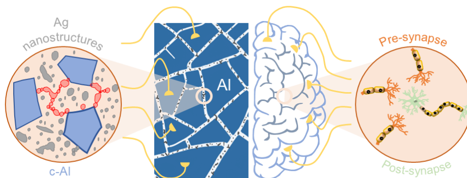
Figure 1. Self-formed hierarchical structures of Al (blue) and Ag (grey) of different length scales (left side), closely mimic the structural hierarchy of biological neural network (right side). Diverse range of Ag filamentary structures (red) show wide ranging synaptic plasticity similar to biological counterpart.
